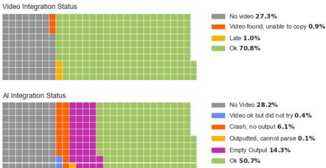
Figure 1. Status of Video (top) and AI (bottom) integration on the edge. 1 block = 100 instances; Each instance occurs at a 5 minute interval.
