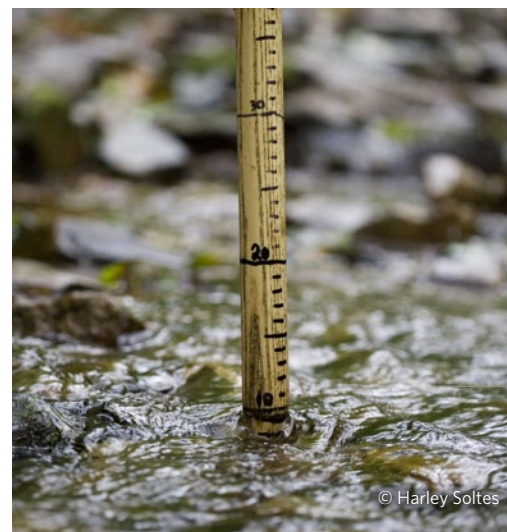
Stream depth measurements are made with a homemade depth gauge, Ellsworth Creek, Willipa Bay, Washington.
