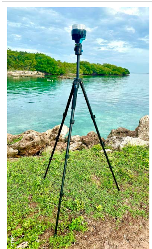
Figure 24. A GNSS base station collecting position correction data during a UAS mission
