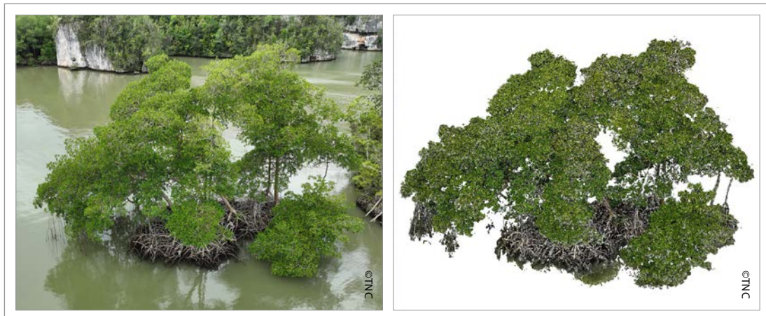
Figure 34. Comparison of the original image of a mangrove and a 3D point cloud 35 generated from stereo images using Agisoft Metashape photogrammetry software
