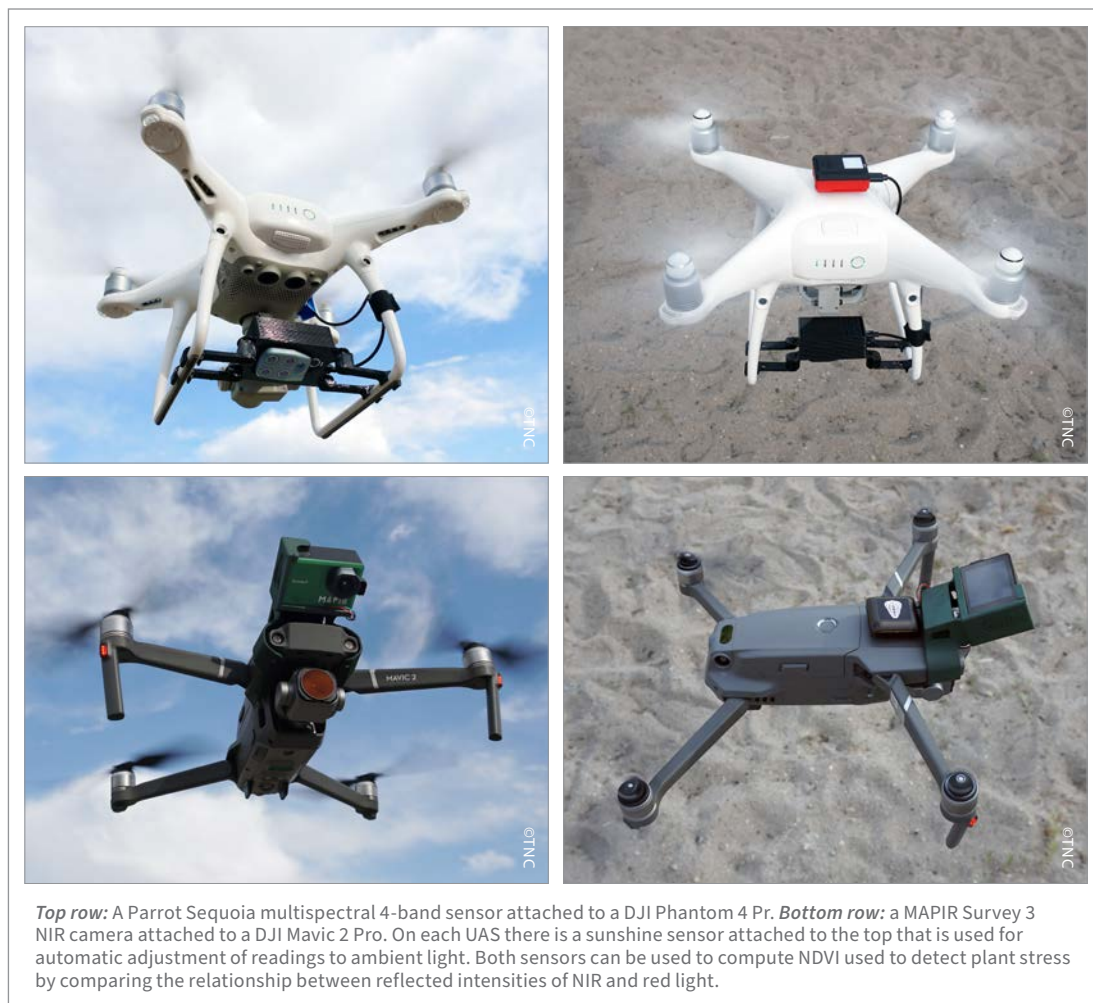
Figure 25. Two cost-effective UAS platforms with supplementary infrared sensors attached for assessing mangrove extent and health
