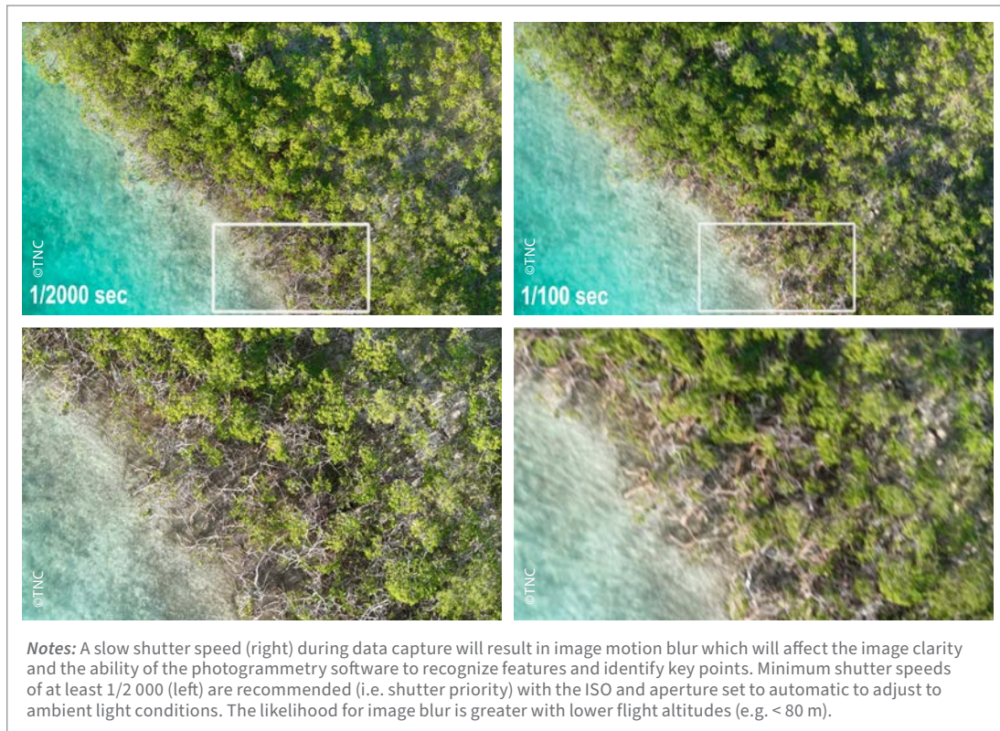
Figure 30. Comparison of UAS images acquired using a fast vs slow shutter speed
