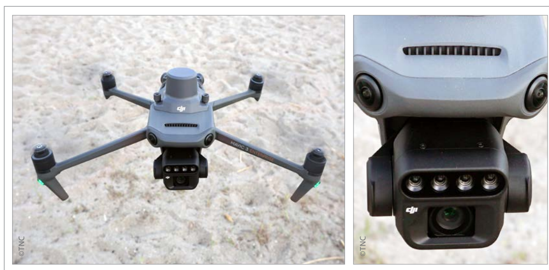
Figure 26. A DJI Mavic 3 Multispectral with a 20 MP RGB camera and integrated 4-band multispectral sensors (green, red, red-edge and NIR) for calculating vegetation indices
